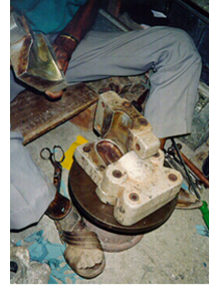
A technician (wearing a below-knee Jaipur prosthesis) reinforcing the rubber in the Jaipur Foot mould before vulcanization.
